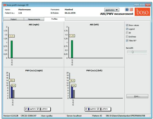
The ABI values (and PWV values if this option is selected) of all measurements are presented in the form of bar charts in the "Profiles" registry. The ABI colour display is as per the setting under "Classification" (red: ABI < 0.9).
